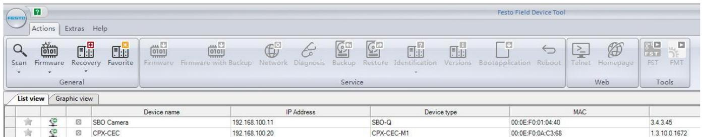
The screenshot shows the Festo Field Device Tool interface. At the top, there are menu options: Actions, Extras, Help. Below the menu is a toolbar with various icons for actions like Scan, Firmware, Recovery, Favorite, etc. The main area displays a table with the following data:
